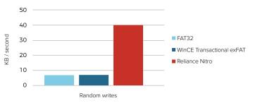
FSIOTest measured the performance of file systems mounted on a PNY 4 GB SD card, producing throughput values for reading from and writing to a file in various patterns. This performance was measured on an i.MX6 Sabre SD embedded board.
